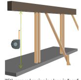
With proper bracing in place in "new" construction, measure the distance from the floor to the header support.
