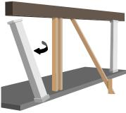
When replacing an existing column, place a temporary support beside the column you are planning to replace. Use a 4x4 or 2x6 and a bottle jack if necessary to make sure the load is properly supported. Once the load is supported remove the old column.
