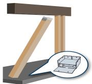
Attach the plinth or metal connector to the bottom of the Culpeper Columns and slide the column into place. If a high wind tiedown cable or rod is required, consult code and manufacturer's recommendations.
