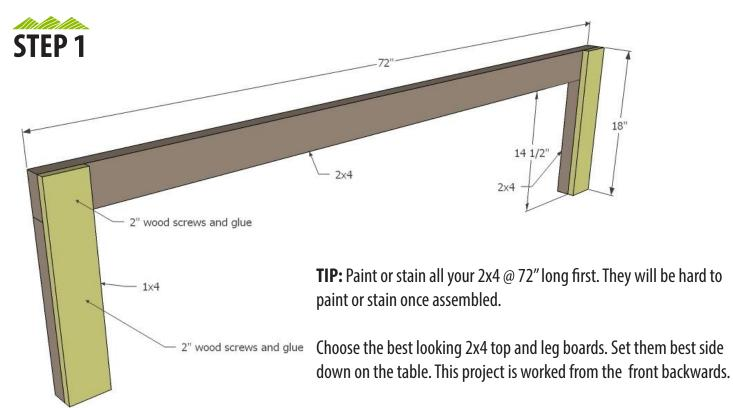
Lay out 1 long 2x4 and 2 short 2x4s. Position the 1x4 on top, apply glue and nail or screw down, to both the top and leg 2x4s.
