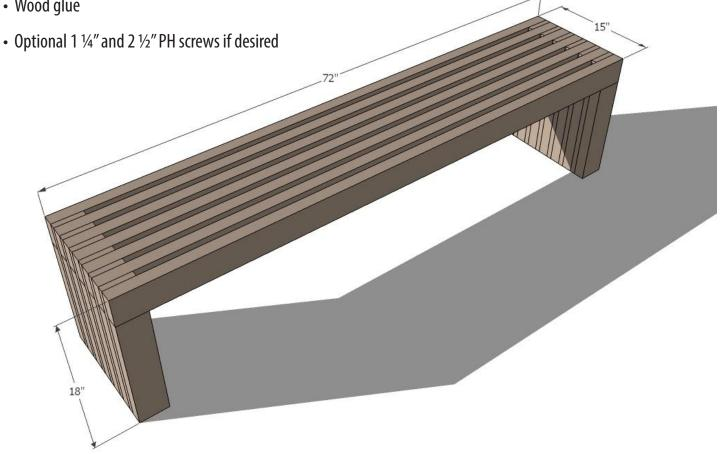
Take all necessary safety precautions. Work on a clean level surface, free from debris. Always use straight boards. Check for square after each step. Always pre-drill holes before attaching with screws. Use glue with finish nails for a stronger hold. Wipe excess glue off bare wood for stained projects, as dried glue will not take stain.
