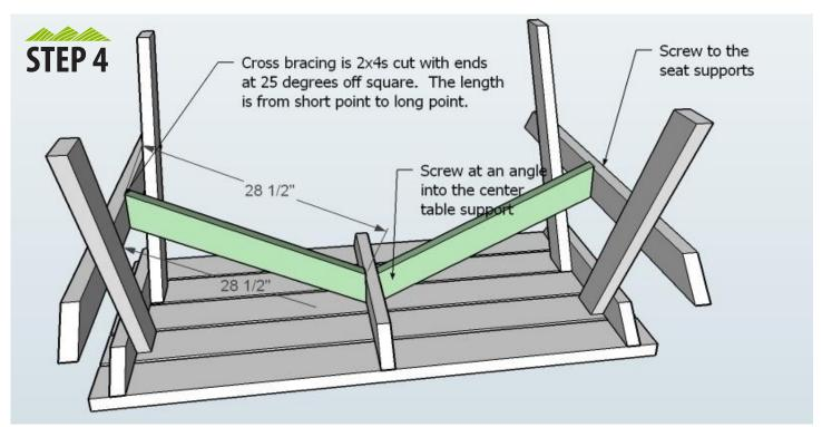
Take a square of the table by measuring from the outer points of the legs to the diagonal opposite leg. Do this for both diagonals. Push the opposite legs together on the longer diagonal until your diagonals match up in distance. Cut cross supports at 25 degrees off square on both ends, (ends are parallel).
