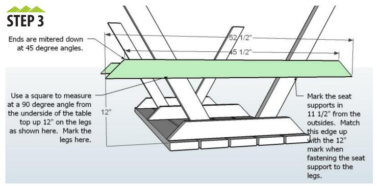
Take square and measure at a 90-degree angle from the underside of the table up 12" and make a mark on the legs. Cut seat supports at 45-degree angles on the ends.
