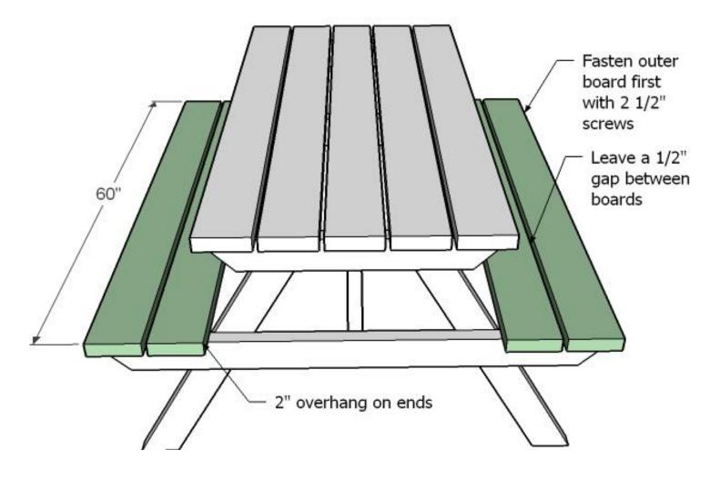
Attach the seat boards to the picnic table with screws to complete.
