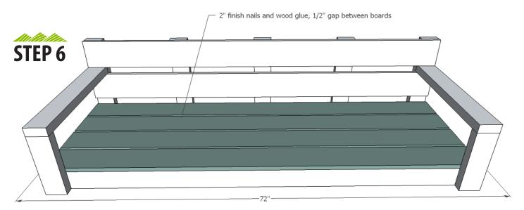
And finally, the seat slats - start at the front, leave 1/2" gaps, and nail and glue down with 2" finish nails.
